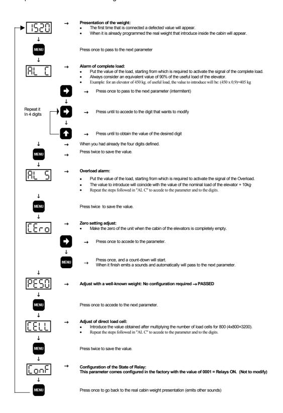
With this quick procedure, we will have perfectly defined the wanted limits of intervention. Our system, starting from now, it will control instantly the load that are introduced in the cabin and it will provide to our controller the necessary data for the load control.
